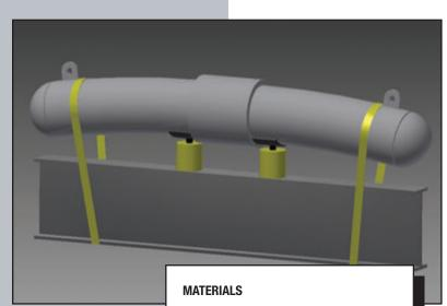
Standard designs are carbon steel, with Pipe Pup metallurgy in API 5L Gr. B and hub/yoke metallurgy in ASTM A105. Also available are Yoke and Hub components in ASTM A694 F42, F46, F50, F52, F56, F60, F65, F70, F80, ASTM A350 LF1, LF2, LF3, LF4, Stainless Steel Grades 304, 304L, 316, 316L, 410, Duplex 311803 and 32750, and special alloys such as Alloy 625 and 825. Pipe Pup metallurgy can be provided to match any available piping materials.
