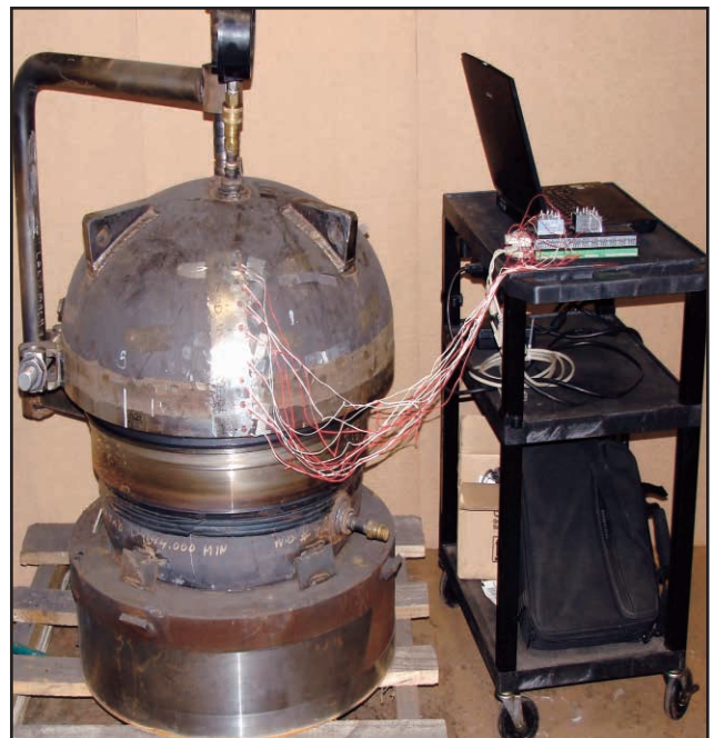
24" CL900V Closure under 3350 psi Hydrostatic Test
